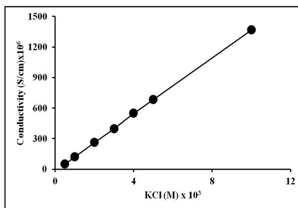
Fig.2. Standard curve for the conductance-meter TEC-4MP
