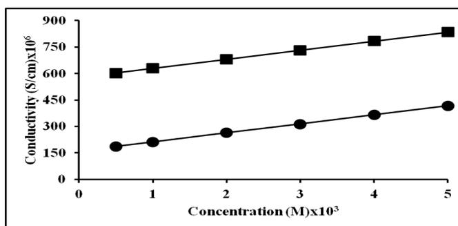
**Fig.4. Conductivity-concentration curves for buffered solutions of NAD at pH 6.5 (●) and 7.5 (■)**
