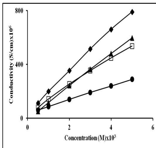
**Fig.3. Conductivity-concentration curves for aqueous solutions of NAD(●), NADP(□), NADH(▲) and NADPH(◆).**
